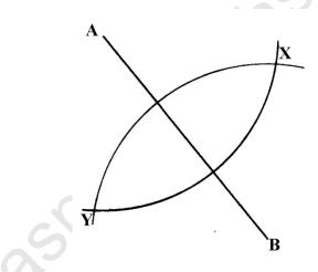
Join X to Y. The line XY is the perpendicular bisector of AB.
