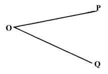
With center O, an arc is drawn to cut OP and OQ at X and Y respectively.
