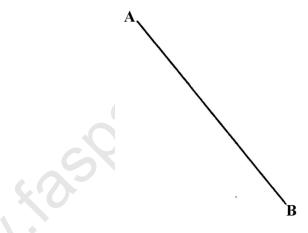
With center A and radius more than half the length of AB, an almost semi-circular arc is drawn.
