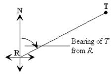
By measurement with the protractor, the angle  $NRT = 65^{\circ}$  $\therefore$  The bearing of T from R is  $065^{\circ}$
