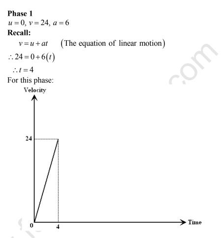
The straight line has a gradient of 6 and indicates a constant acceleration of 6 ms<sup>-2</sup>.
